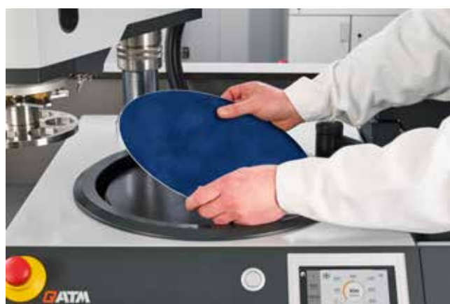
Placing e.g. a GALAXY polishing cloth on the magnetic foil
