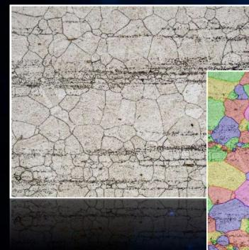
Al capabilities can automatically and correctly segment grains even on scratched or similarly damaged samples.
