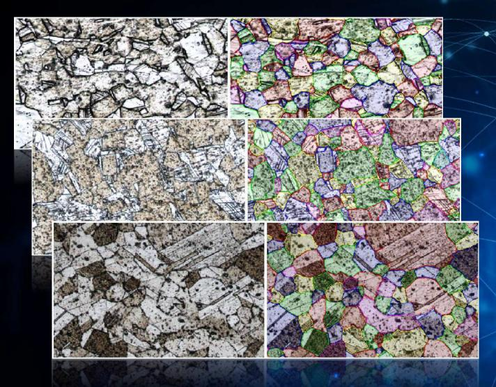
Reliable AI grain detection currently works primarily on Austenitic and Ferritic one-phase structures.
