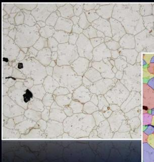
Grain detection using AI in NIS-Elements properly segments grains on images containing various interfering particles or defects.
