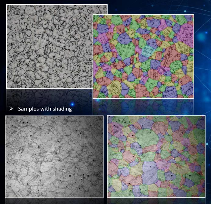
Al network is trained to correctly identify individual grains also on the images with shading. Achieving such excellent results is very difficult using common segmentation methods.
