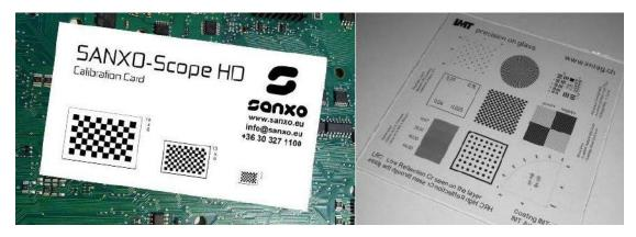
You can have your own calibration card. The setup supports adding a new calibration pattern, so if you go for higher magnification just print your new calibration card and you can use it directly. The calibration card is used for high accuracy. Its resolution is 0.015 micron. At ca. 140x magnification the 1-micron measurement accuracy can be achieved.
