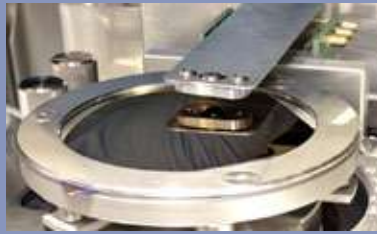
Ball on disk setup for nanotribology agglomerated particles on a coating.
