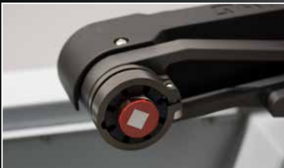
Rotating device with reducing ring for embedded samples
