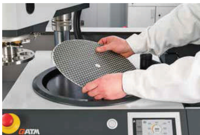
Placing e.g. a diamond grinding disc on the magnetic foil
