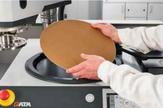
Applying GALAXY X-Tap on magnetic foil
