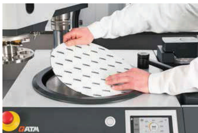
Applying the adhesive carrier disc
