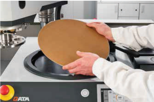
Applying GALAXY X-Tap on magnetic foil
