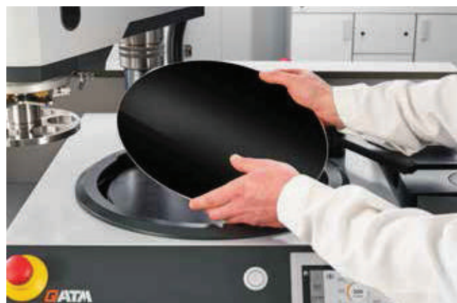
Applying GALAXY Quick-Tap on magnetic foil
