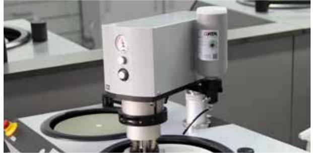
The Qdoser ONE dosing system is an easy-to-use solution for manual or semi-automatic polishing processes. QATM's standard suspension and lubricant bottles can be quickly screwed on the dosing attachment. The dosing volume is closely
